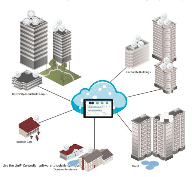
administer an enterprise Wi-Fi network – no special training required. RF map and performance features, real-time status, automatic UAP device detection, and advanced security options are all seamlessly integrated.
