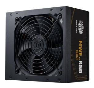
Introducing the MWE Bronze V3, the evolutionary next step in Cooler Master power and the ATX 3.1 upgrade to our MWE Bronze V2 PSU. With features such as 80 Plus Bronze efficiency, a DC-to-DC + LLC circuit design, and a quiet HDB fan cooling, the V3 provides valuable performance in multiple dimensions.
