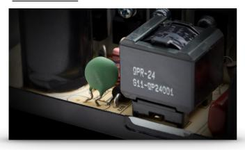
XPG PROBE 500's varistor acts as a control element to offer optimal operating condition, and it protects the PSU from excessive transient voltages.
